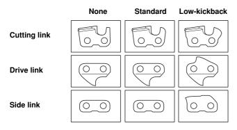
Combining these links in different ways gives different degrees of kickback reduction. In terms of kickback reduction alone, four different types of link are available.
